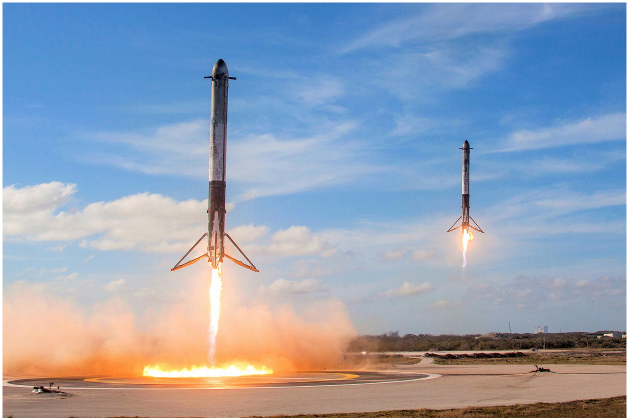
Figure 1: SpaceX Falcon 9 rockets using propulsion to slow their descent (From SpaceX on Flickr)
